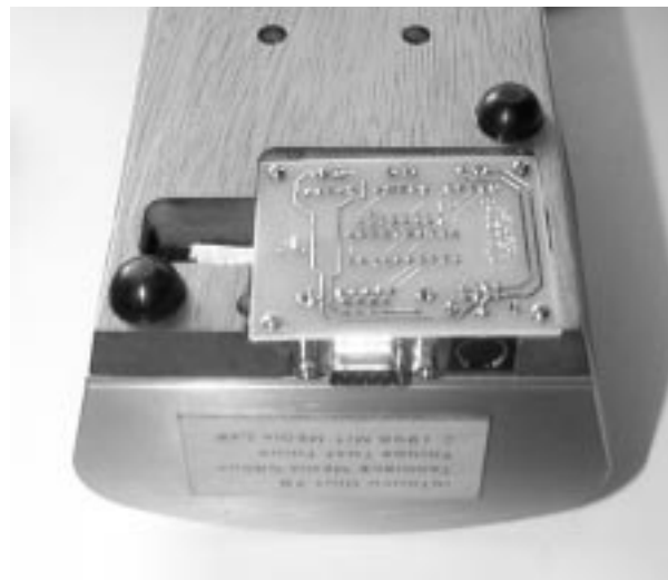
Figure 5.4: Auxiliary board mounted to the mechanical unit
